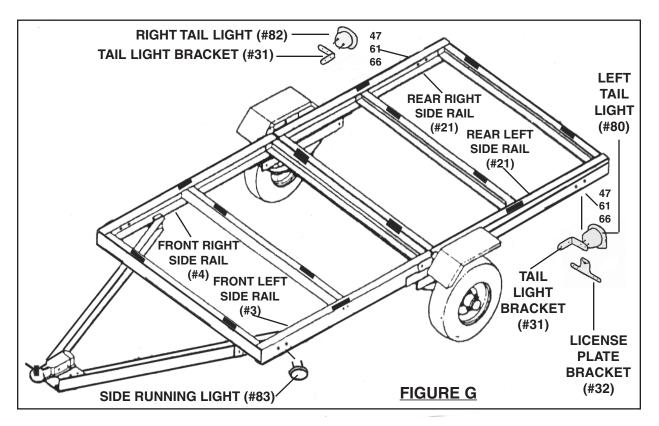
20. To install the Wiring Harness (part #84), temporarily loosen one Bolt (part #47) that is located on the Coupler (part #1). To ground the Wiring Harness, bare about 1" of the end of the White Ground Wire to expose its copper strands. Wrap the exposed copper strands around and under the head of the loose Bolt. Then, retighten the Bolt.
